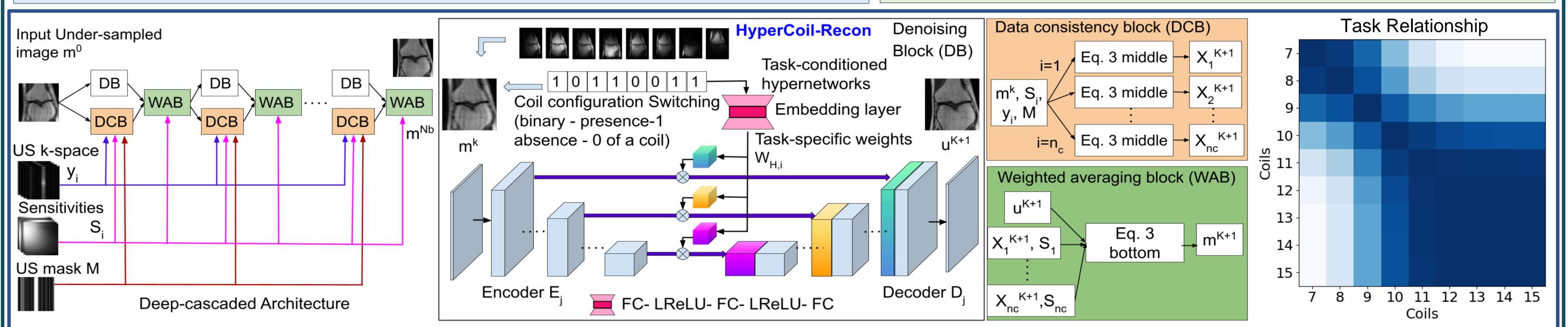
Fig 2: (Left) Deep Cascaded HyperCoil-Recon Architecture with the hypernetwork blocks, data consistency, and weighted-average blocks. The hypernetwork has three fully connected layers and two Leaky ReLU non-linear layers. (Right) Matrix plot showing the inter-task relationship. Tasks with neighboring coil configurations exhibit more similarity, while far-apart configurations exhibit lesser similarity.
